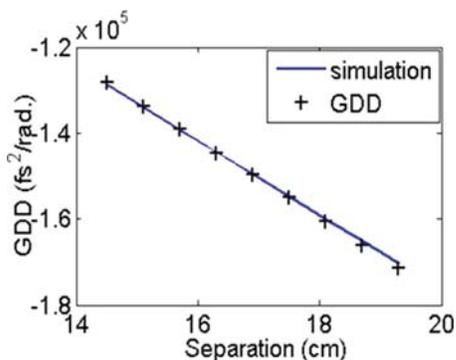
Fig. 6. (Color online) Variation of GDD versus distance in single-grating pulse compressor.
