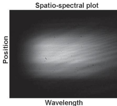
Fig. 8. Spatio-spectral plot revealing the lack of spatial chirp in the compressor output after four beam passes, indicated by the lack of tilt in this plot. The minor structure and the fringes at right are due to a stray reflection also entering the spectrometer and hence are of no significance.
