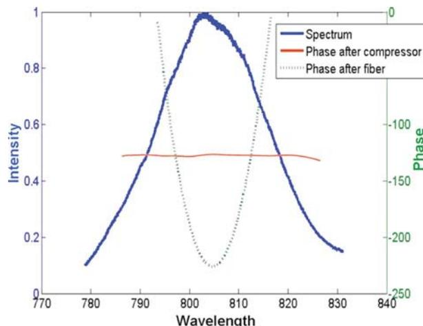
Fig. 9. (Color online) Spectrum and spectral phase before and after the compressor.
