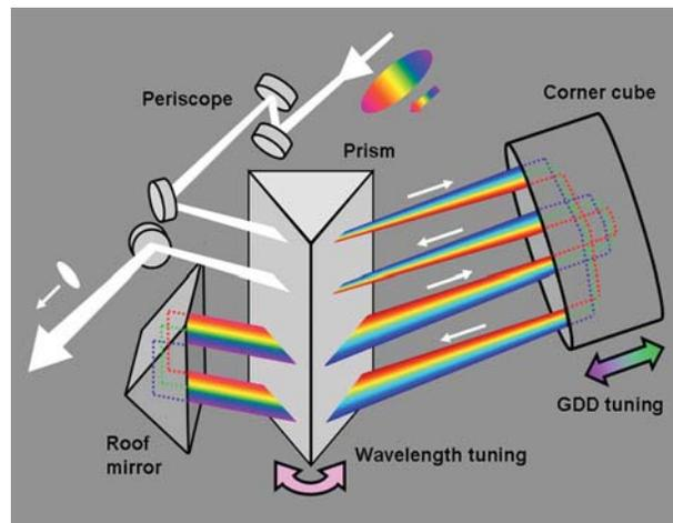
Fig. 3. (Color online) Schematic diagram of single-prism pulse compressor.
