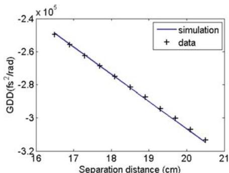
Fig. 7. (Color online) GDD versus distance in single-grism pulse compressor.
