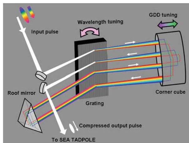
Fig. 4. (Color online) Schematic diagram of single-grating pulse compressor.
