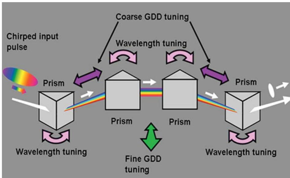
Fig. 1. (Color online) Conventional four-prism pulse compressor.
