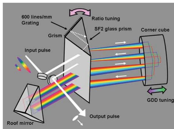
Fig. 5. (Color online) Schematic diagram for single-grism pulse compressor.
