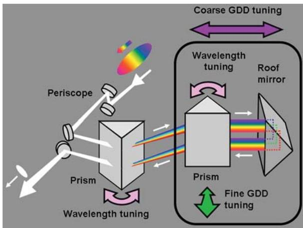
Fig. 2. (Color online) Two-prism pulse compressor.
