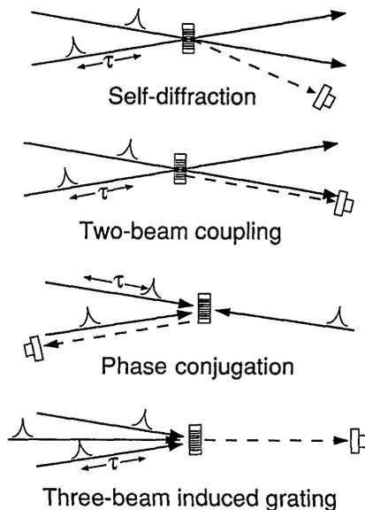
Fig. 1. Various beam geometries for performing IGA. Both three-beam geometries are essentially equivalent for this purpose.
