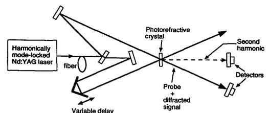
Fig. 5. Experimental apparatus, a standard photorefractive-beam-coupling arrangement, but with SHG possible simultaneously.
