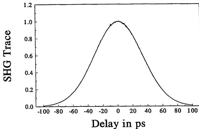
Fig. 6. Simultaneous SHGA measurement made with the same apparatus and crystal as in photorefractive-beam-coupling IGA measurements.
