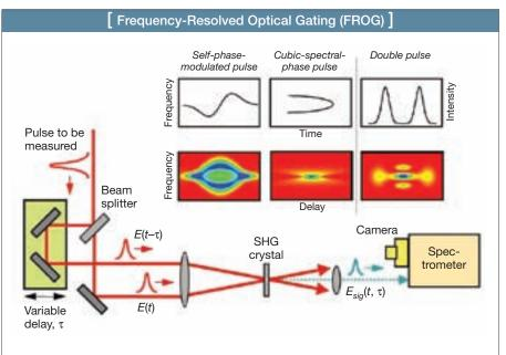
FROG: a spectrally resolved autocorrelation. Two pulse replicas cross in a secondharmonic (SH) generation or other nonlinear medium, and the SH spectrum is measured vs. the pulse relative delay. FROG yields the pulse intensity and phase vs. time (and frequency). Upper right: FROG traces (below) for some pulses (above).
