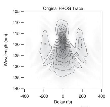
FIGURE 3 POLKADOT FROG Trace. This is the  $\sqrt{I_{\rm FROG}}$  of an SHG FROG trace using a 50% / 10% etalon as a beam splitter as described in the text
