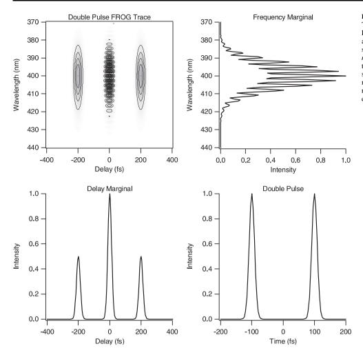
FIGURE 2 Double Pulse FROG Trace. This figure shows the SHG FROG trace for two 20-fs pulses separated by 200 fs (The pulse train is shown in the *lower right-hand corner*.) The trace in the *upper left* shows the square root of the FROG intensity, *I*<sub>FROG</sub>. Also shown are the two marginals (integrals if the trace with respect to delay or frequency) that exhibit characteristic modulations
