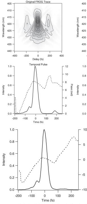
**FIGURE 9** The Retrieved Pulse Correction. The pulse after subtracting off the trailing pulses as described in (5). The secondary pulse is completely gone
