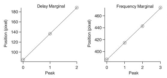
FIGURE 6 Peak Positions and Calibration Fit Functions. Shown here are the peak positions from the marginals and the straight line fits. The delay marginal fit was 84. +951x, and the frequency marginal fit was 38 + 628x, where x is the peak number
