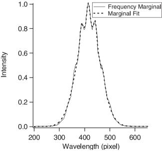
**FIGURE 5** Frequency Marginal (equal to the autoconvolution of the spectrum). The frequency marginal has peaks separated by the reciprocal of the pulse separation. The fit of Function (1) to the marginal is also shown
