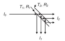
**FIGURE 10** Etalon Schematic. This is an exaggerated diagram of an etalon. The input beam,  $I_0$ , bounces between the two partially surfaces. Each round trip creates an attenuated, delayed replica of the input pulse
