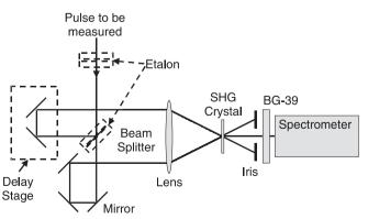
FIGURE 1 FROG Device Schematic. A schematic layout of an SHG FROG device, showing two possible positions for the etalon in the POLKADOT FROG arrangement, both of which automatically calibrate the device and remove the ambiguity in the direction of time
