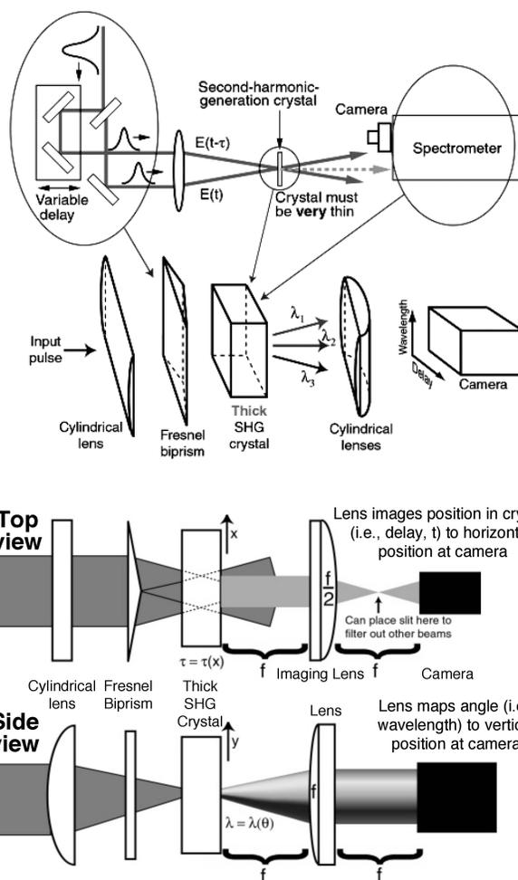
Fig. 1. (Top). A FROG device (above) and its simpler version, GRENOUILLE (below). (Bottom) Top and side views of GRENOUILLE.
