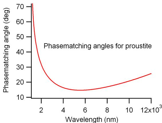
Fig. 6. Phase-matching curve for Proustite. Proustite also begins to absorb very strongly below 600 $\mu\text{m}$ .
