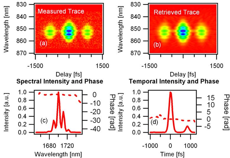
Fig. 4. Tests of our 1.5- $\mu\text{m}$  GRENOUILLE with more complicated pulses: (a) Measured and (b) retrieved GRENOUILLE traces (FROG error 0.0055) for a double pulse; (c-d) retrieved spectral and temporal intensity and phase.
