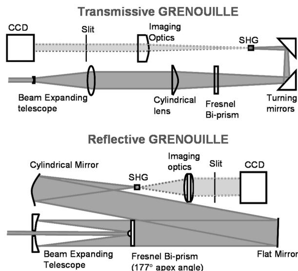
Fig. 1. Compact GRENOUILLE geometries. Previous transmissive design for measuring pulses as short as 50 fs (top) and reflective GRENOUILLE design for measuring ~20-fs pulses (bottom).
