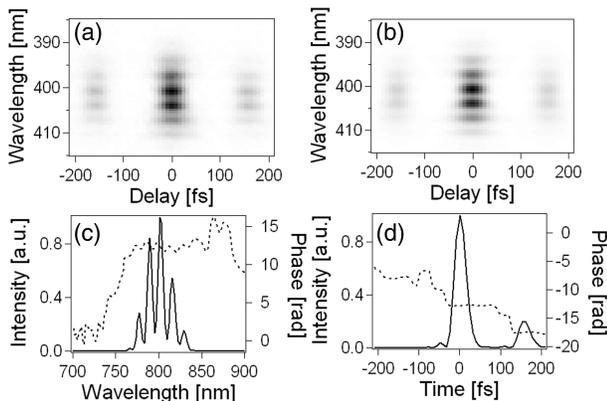
Fig. 4. (a) Measured and (b) retrieved GRENOUILLE traces (FROG error of 0.00643) for a double pulse. Note the characteristic fringed double-pulse trace. (c) Spectrum and spectral phase and (d) intensity and phase versus time for a double pulse.
