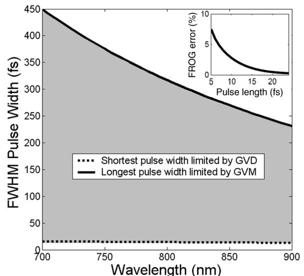
Fig. 2. Pulses measurable by use of GRENOUILLE with a 1.65-mm BBO crystal. The solid curve represents the (upper) limit set by the spectral resolution of the crystal ( $L \times \text{GVM} = \tau_p$ ). The dashed curve represents the (lower) limit set by the GVD induced by the crystal [ $(L/2)\text{GVD} = \tau_c$ ]. Inset, theoretical FROG error versus pulse width due to crystal dispersion.
