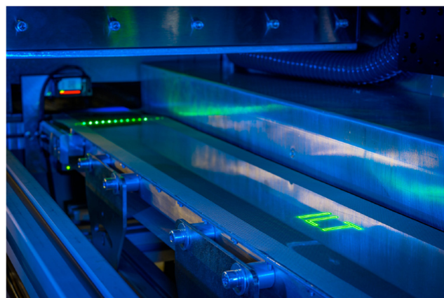
Figure 4. (Top) NCF for delivering ultrashort pulses [32]. (Bottom) Parallel ultrafast LMP of organic solar cells. (Reproduced courtesy of Dr-Ing. Arnold Gillner.)
