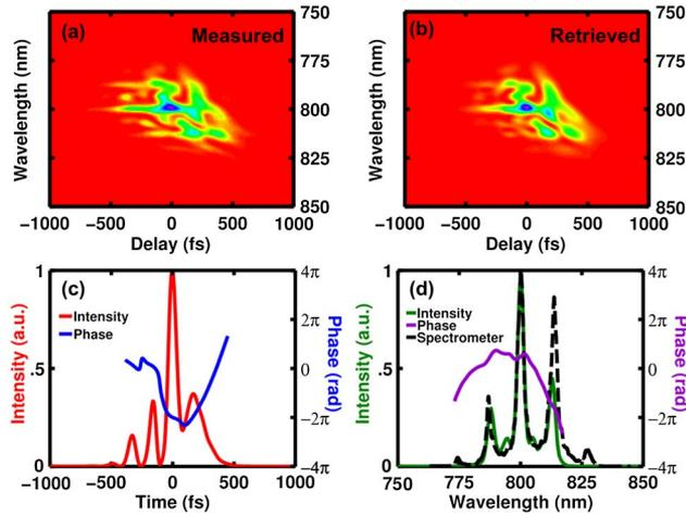
Fig. 4. (Color online) (a) Measured trace 1 for a chirped pulse train; (b) Retrieved trace 1 with a FROG error of 0.81%; (c) Retrieved pulse intensity and phase in temporal domain showing structures from chirped pulse beating; (d) The measured spectrum and the spectral phase compared with measurement made by a spectrometer.
