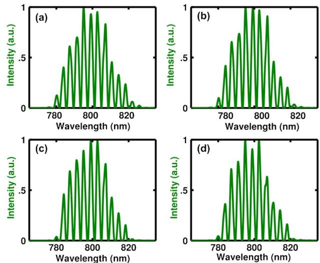
Fig. 10. (Color online) Four spectra of the same pulse measured at different times. The spectra have same fringes separation but a slightly different envelope.
