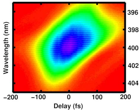
Fig. 11. (Color online) Higher resolution plot of the DB PG FROG trace captured in the 400 nm arm showing the higher frequency fringe artifact due to etalon effects in the nonlinear medium.
