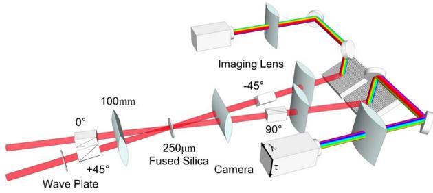
Fig. 1. (Color online) Schematic of single-shot DB PG FROG for measuring an unknown pulse pair.
