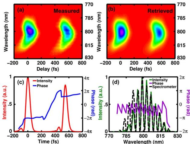
Fig. 9. (Color online) (a) Measured DB PG FROG trace for a well separated double pulse at 800 nm; (b) Retrieved trace with a FROG error of 0.52%; (c) Retrieved pulse intensity and phase in temporal domain; (d) The measured spectrum and the spectral phase compared with a measurement made by a spectrometer.
