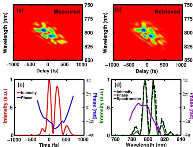
Fig. 5. (Color online) (a) Measured trace 2 for a chirped double pulse; (b) Retrieved trace 2 with a FROG error of 0.74%; (c) Retrieved pulse intensity and phase in temporal domain showing structures from chirped pulse beating; (d) The measured spectrum and the spectral phase compared with measurement made by a spectrometer.
