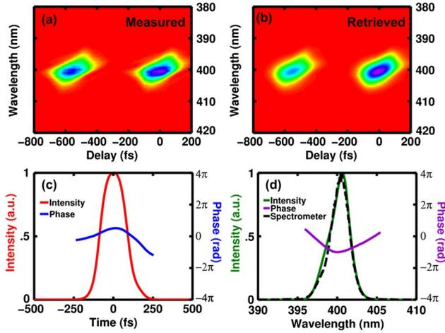
Fig. 8. (Color online) (a) Measured DB PG FROG trace for a simple pulse at 400 nm; (b) Retrieved trace with a FROG error of 0.83%; (c) Retrieved pulse intensity and phase in temporal domain; (d) The measured spectrum and the spectral phase compared with a measurement made by a spectrometer.
