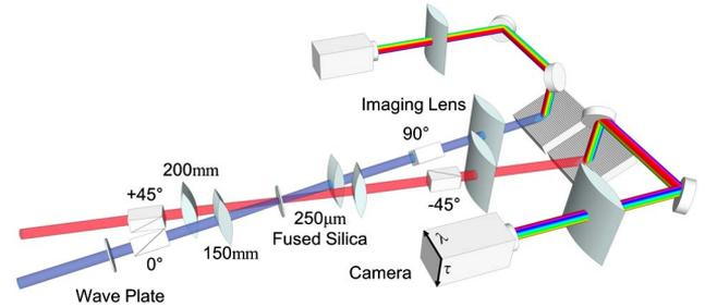
Fig. 3. (Color online) Schematic of single-shot DB PG FROG for measuring an unknown pulse pair at different wavelengths (400 and 800 nm in our experiment).
