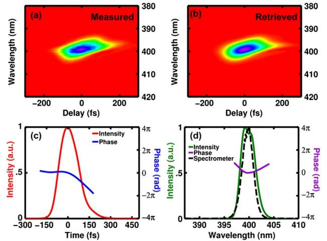
Fig. 6. (Color online) (a) Measured trace for a simple pulse at 400 nm; (b) Retrieved trace with a FROG error of 0.32%; (c) Retrieved pulse intensity and phase in temporal domain showing structures from chirped pulse beating; (d) The measured spectrum and the spectral phase compared with measurement made by a spectrometer.
