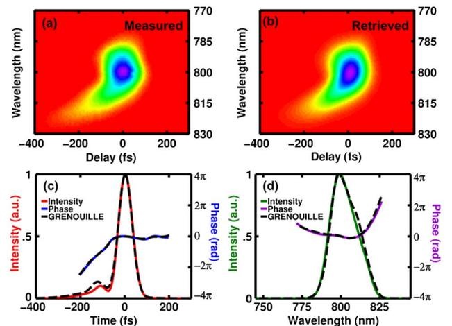
Fig. 7. (Color online) (a) Measured trace for a simple pulse at 800 nm; (b) Retrieved trace with a FROG error of 0.30%; (c) Retrieved pulse intensity and phase in time compared with an independent GRENOUILLE measurement; (d) The measured spectrum and the spectral phase compared with those made using a GRENOUILLE.
